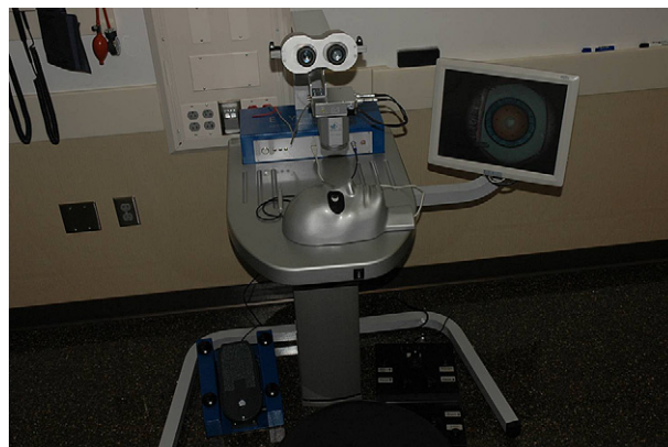
Figure 1. EYESi surgical simulator. Note left multifunctional phaco and vitrectomy foot pedal, right microscope pedal, and right touch screen instructor control and viewing display. The virtual operating microscope has a stereoscopic view with interchangeable “cataract head” hardware, shown here on the adjustable platform.
